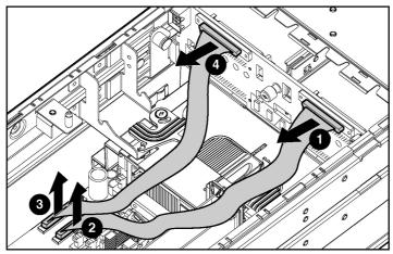
Figure 1-10: Disconnecting the SCSI cables
